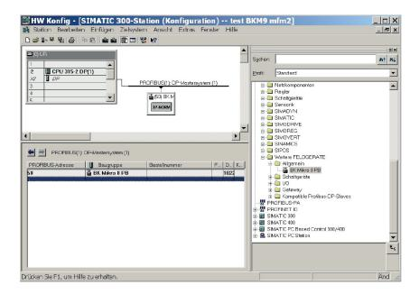
3. Allocate the correct Profibus address of the module.
